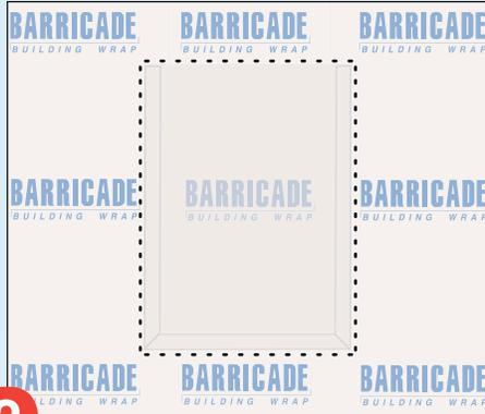
**2** Secure Barricade® firmly in place by fastening it every 12"–18" along the vertical studs using large-headed or plastic cap nails or minimum 1" crown staples. You may install it over wood based, foam insulative, or fiberboard sheathing, and exterior gypsum board.
