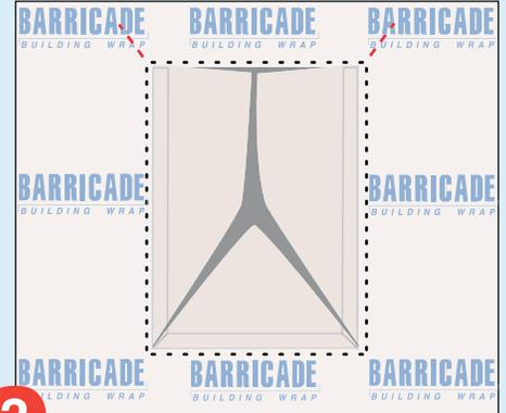
**3** Make an inverted Y cut in the wrap at window rough opening. Make diagonal cuts at the top of the rough opening corners.
