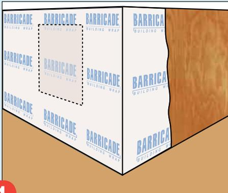
**1** Start 2–3 feet from a corner. Wrap around corner and continue nailing or stapling as you move around the house. Use fasteners that are long enough to penetrate into the stud or nail base material.
