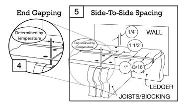
Note: Special consideration should be taken when working with dark colors as they will experience larger temperature swings during normal use. To help control end-to-end spacing, dark color decking should be kept at ambient temperature and shaded from direct sun prior to cutting and immediate securing.
