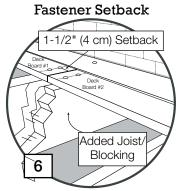
Screw heads must be flush with board surface. Use caution to avoid over-tightening fasteners. Excess tightening may cause immediate or eventual cracking of the fastener locations.
