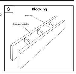
When installing blocking for more intricate decking patterns, remember that solid blocking (blocking laid on the flat) will inhibit water flow and result in buildup of organic materials over time, which will make cleaning more difficult. For best results when blocking is required, it should be installed ladder style (Figure 3).
